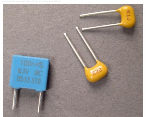
Caps come in many shapes and flavors. A good rule of thumb for the novice is when you're looking at some circuit or other and you can't tell what some component is, it's probably a cap. These particular caps are examples of "film caps" and "ceramic caps". Both are higher in quality and lower in capacitance (measured in FARADS) than their big electrolytic cousins, and they aren't polarized, so you can stick them in the board any old way you want.
