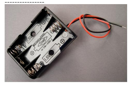
Holds the batteries. I'm trying very hard to think of something smart to say about this part, and coming up challenged. How about this: "Put the batteries in the same way as in the picture!" or "The red lead is positive (connects to V+) and the black lead is ground," or "The battery holder comes pre drilled for 4-40 screws, but make sure those screws have a countersink!"
