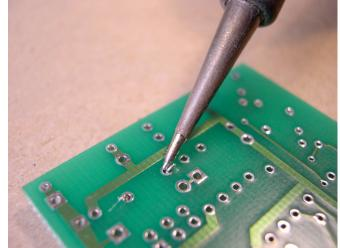
Next, with your other hand, apply solder to the junction of the component lead and pad. Here are some action shots:
