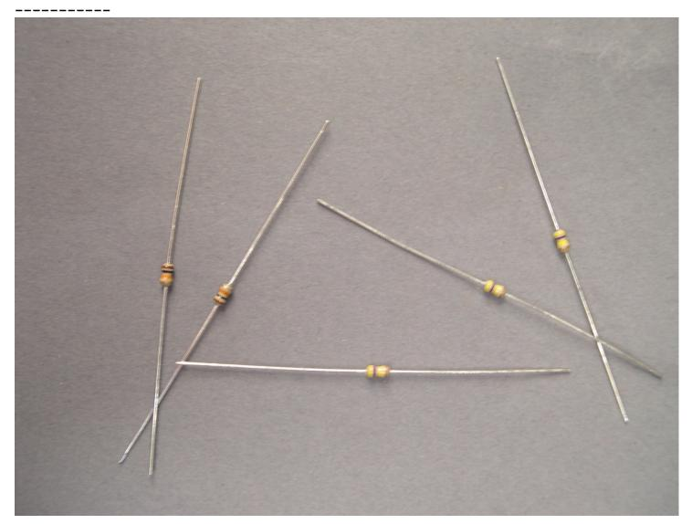
Resistors are the little workhorses of electronics. They usually consist of carbon or metal film, and they essentially oppose the flow of current. Resistors are used to divide voltage, limit current, make noise sources, and are
