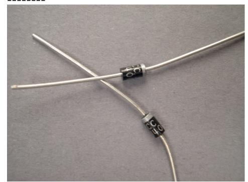
Diodes are one-way gates for current, and as such are polar. In this kit, the diodes handle protecting the inputs from overvoltages and protecting the kit
