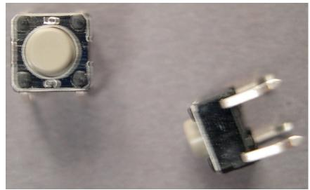
An unexciting but necessary component for user interface. These are called "tact switches" I guess because you can feel them. Switches either make a connection or break one when you press the button. In this case, they make one (they are "Normally Open") and they only make it while the button is held down (they are "Momentary").
