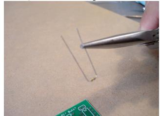
Now, insert the resistor in its proper spot on the board. Push it all the way down until it looks like this:
