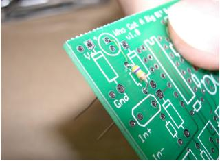
Keeping your finger on top of the resistor so that it doesn't fall out, turn the board over and bend the leads so that the resistor can't fall out. It should look like this:
